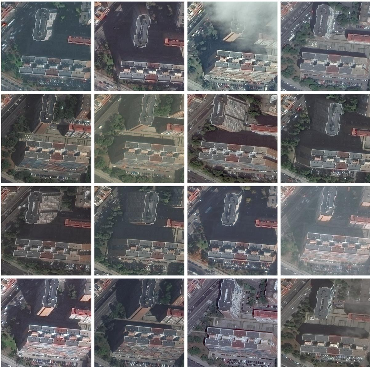
Figure 3.2: Challenging appearance variability due to different factors including viewpoint changes (nadir angle), shadows, daylight changes marked by weather and seasons, etc.
