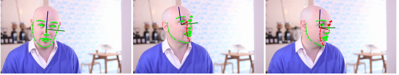
Fig. 1: Simultaneous head pose estimation, facial landmark location and their visibility predictions when processing a video from 300VW [14]. Green and red points show visible and non-visible landmarks respectively. The co-ordinate system qualitatively represents head pose.
